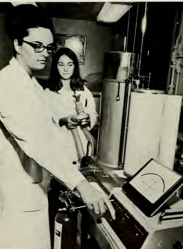
Lab technician Patty Griffin checks the inhalator which measures pollution content of the air, as technician Georgia Weaver takes a reading on the same machine.
